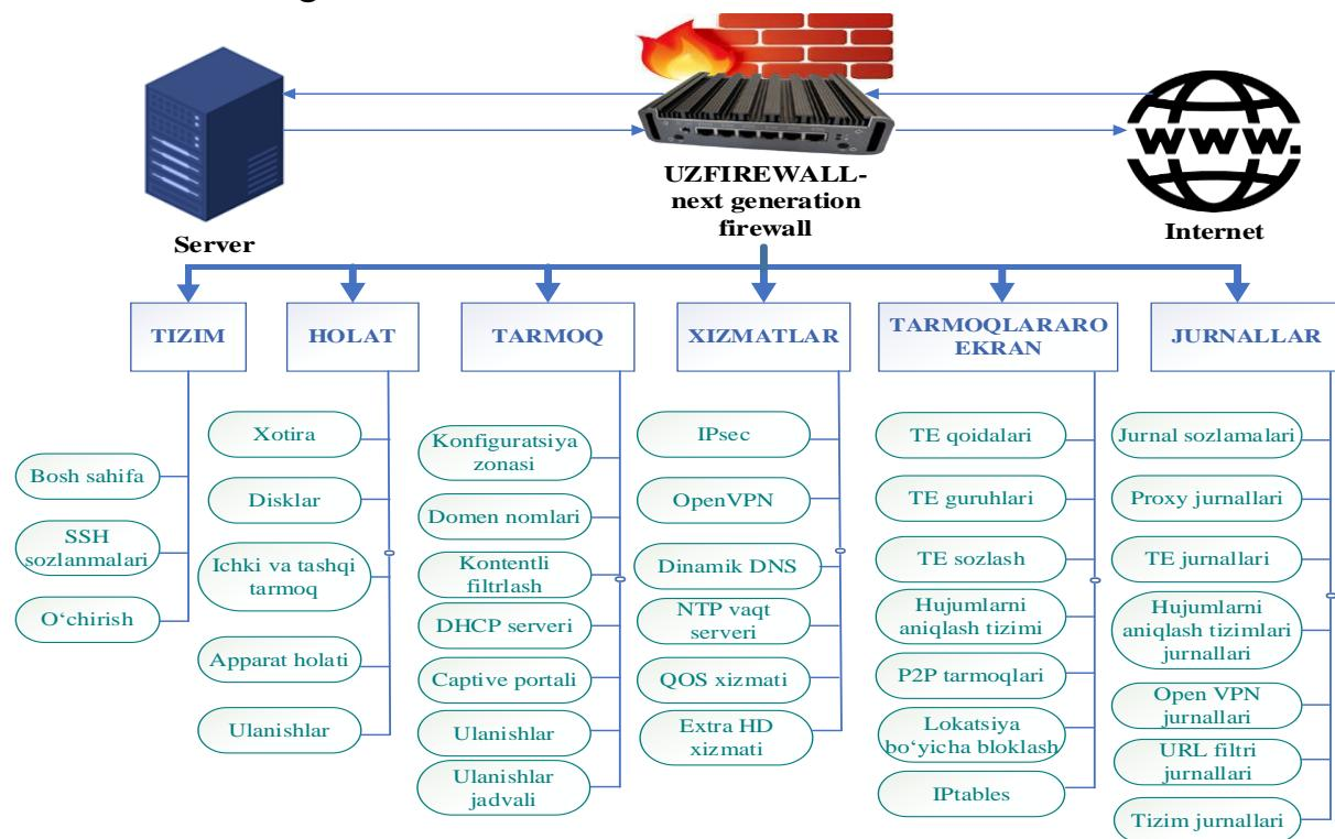
**7-rasm.** UzFirewall-next generation firewall apparat-dasturiy vositasining umumiyligini funksional strukturasi
